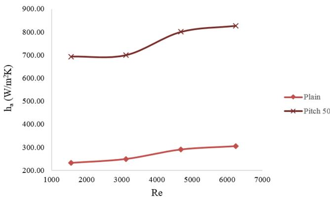
Figure 8.  $h_a$  vs Re for 50 mm pitch
