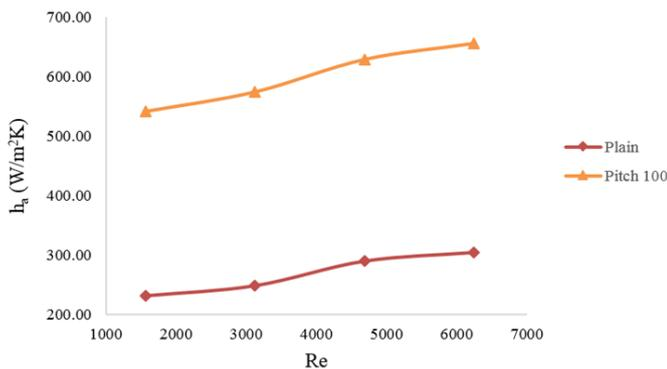
Figure 7.  $h_a$  vs. Re for 100 mm pitch
