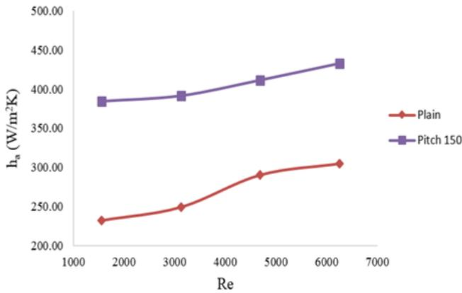
Figure 6.  $h_a$  vs. Re for 150 mm pitch
