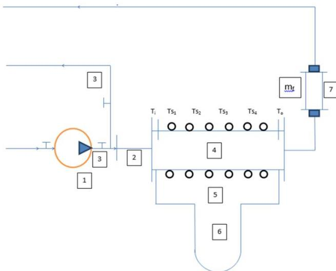
Figure 2. Experimental Setup. (1) Pump, (2) Calming Section, (3) Flow control section, (4) Test Section, (5) Electric Heater, (6) Manometer, (7) Rotametr
