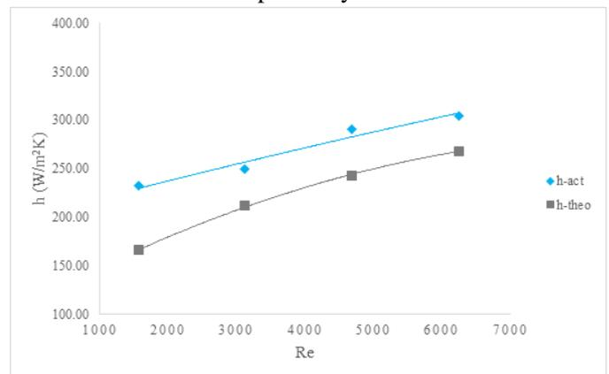
Figure 5.  $h_{th}$  &  $h_a$  vs. Re for plain tube
