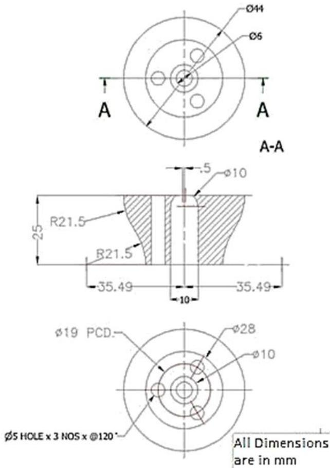
Figure 1. Production drawing of swirl flow insert
