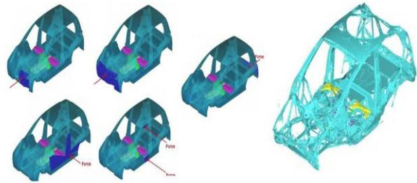
**Figure 2:** Equivalent static loads and optimization result for the Future Steel Vehicle.
