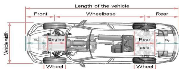
**Figure 4:** Free crash lengths  $s_f$  and  $s_r$  (simplified).
