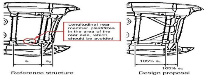
**Figure 12:** Performance of the optimized topology compared to the reference design.
