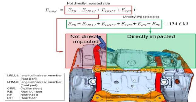
Figure 6: Main vehicle parts for the offset rear impact.
