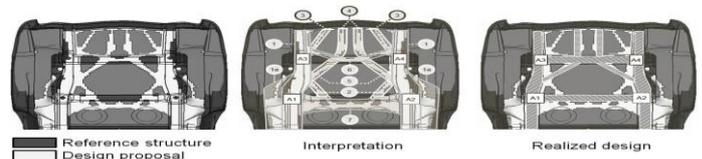
**Figure 11:** Optimized topology compared to the reference design and its interpretation.
