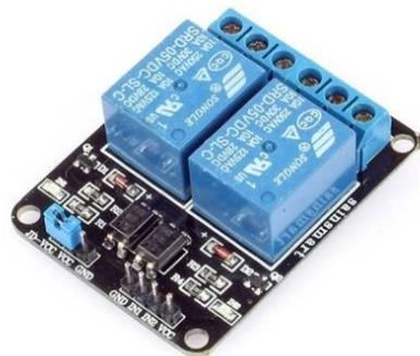
**Figure 4: Relay Module**
