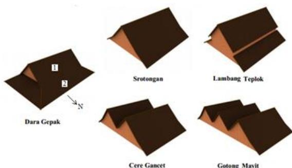
**Figure 3:** The roof model of Javanese village house (1. Gajah, 2. Emper) [20]
