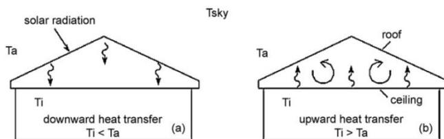
**Figure 1:** Kind of heat transfer in a roof [8]
