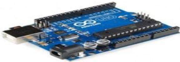
**Figure 5:** An Arduino Uno Board
