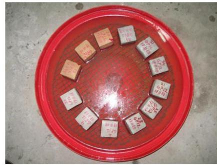
Figure 1. Setup for water sorptivity test
