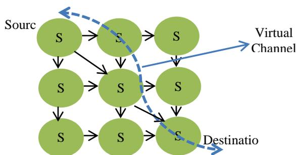
Figure 4, 3x3 NoC switch and their direction with virtual channel
