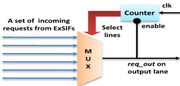
Figure 5: Distributed round-robin arbiter architecture for one output lane.
