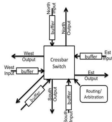
**Figure 1:** Typical Router architecture with five input and output ports (north, east, south, west and local).
