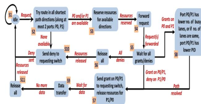
Figure 7: State diagram for a switch's channel phase actions and transitions
