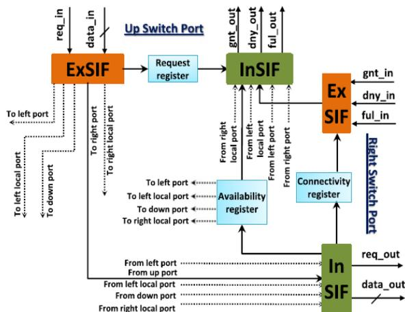
Figure 3: A subset of internal connection between the signal forwarders (ExSIF and InSIF) and status register placement for two arbitrary lanes (up and right).
