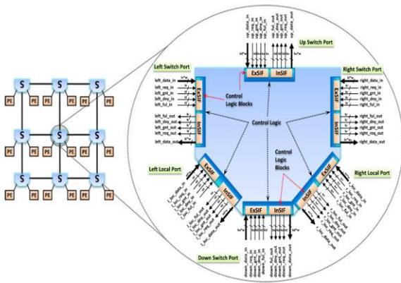
**Figure 2:** 3 x 3- MACS's architectural layout (left) and detailed MACS switches architecture (right).
