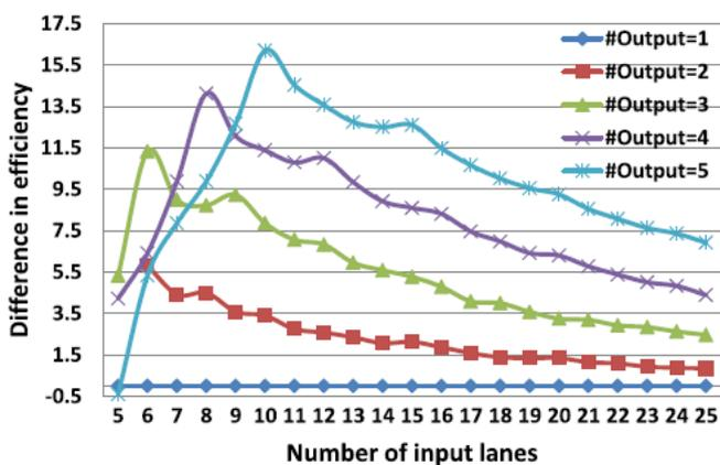
Figure 6: The percentage efficiency difference between the typical and distributed round robin arbiters
