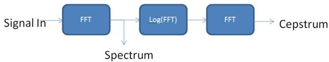
**Figure 2.** Block diagram of Cepstrum Coefficient Calculation
