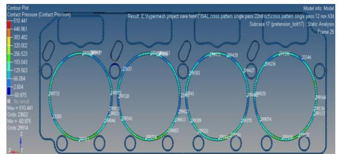
**Figure 10.** FEA results of Contact Pressure distribution on gasket elements
