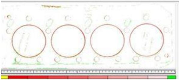
**Figure 11.** 11 High Pressure Fuji-film results on the gasket
