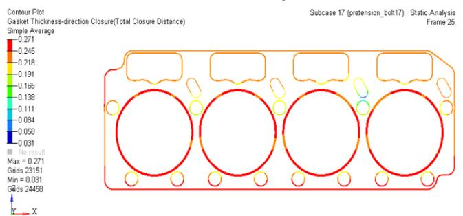
**Figure 7.** Gasket Thickness direction closure (in mm) for the various bead areas of the gasket.
