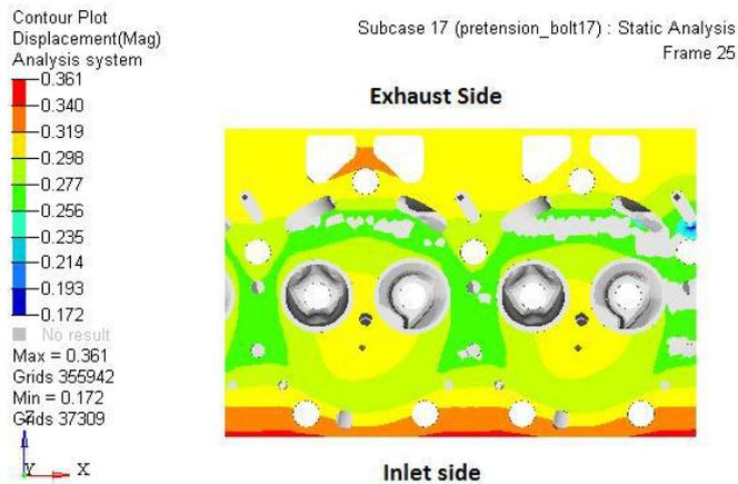
**Figure 8.** Head Deck Surface deformation
