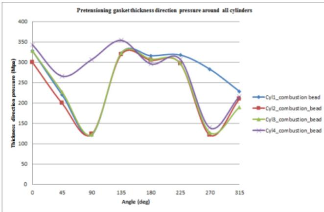
**Figure 4.** Comparison of gasket thickness direction pressure around Cylinders 1, 2, 3 & 4 in combustion bead area
