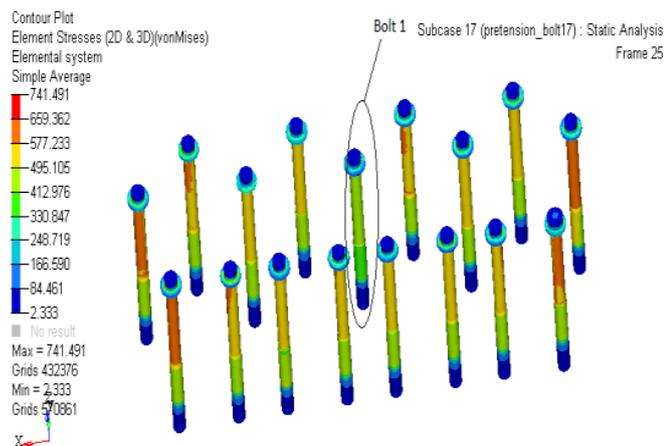
**Figure 9.** Bolt 3D stresses (von-mises) in Mpa
