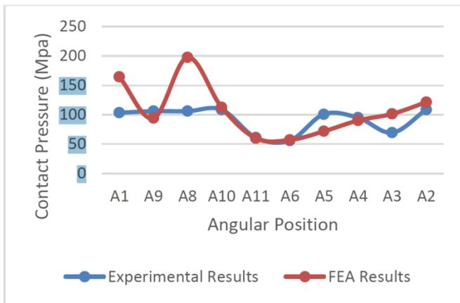
Comparison of contact pressure at cylinder 1 combustion bead
