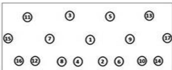
Figure 2. Cross bolt tightening pattern
