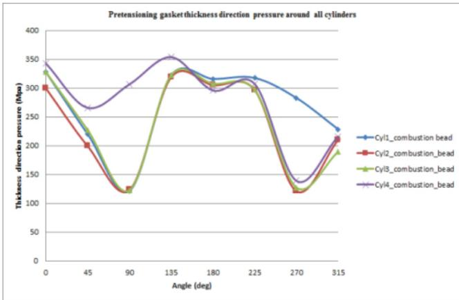
**Figure 4.** Comparison of gasket thickness direction pressure around Cylinders 1, 2, 3 & 4 in combustion bead area
