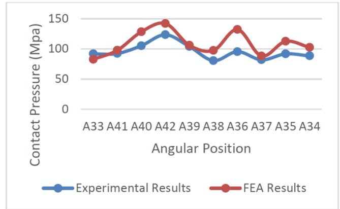
Comparison of contact pressure at cylinder 4 combustion bead
