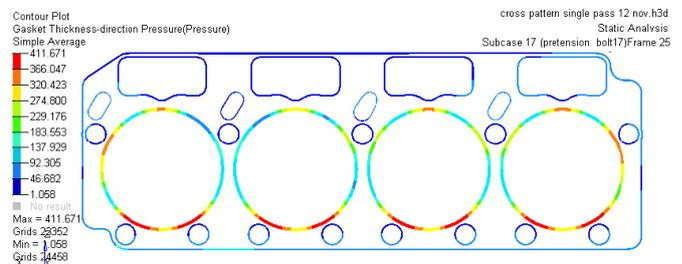
Figure 3. Gasket Thickness direction pressure (MPa) for the various gasket bead areas.
