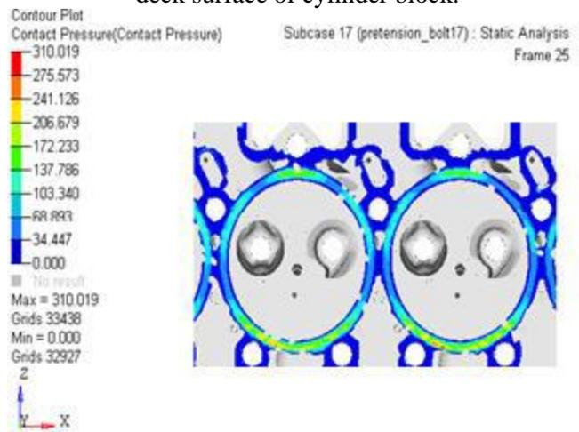
**Figure 6.** Contact pressure distribution (in Mpa) on bottom deck surface of cylinder head.
