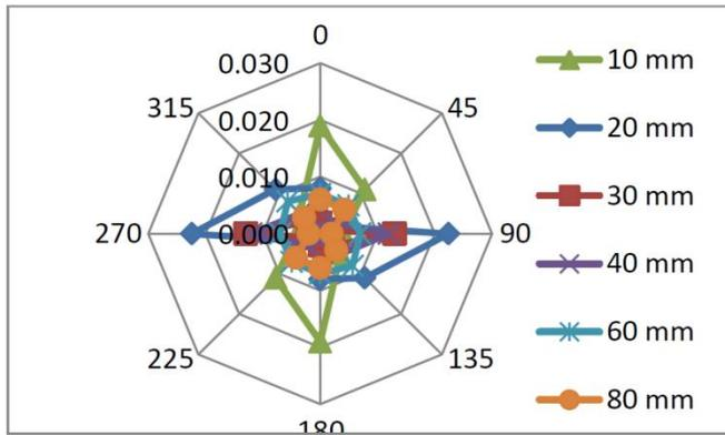
**Figure 13.** Bore Deformation because of cross pattern at different liner height
