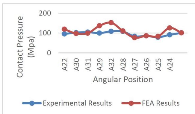
Comparison of contact pressure at cylinder 3 combustion bead
