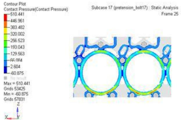
**Figure 5.** Contact pressure distribution (in Mpa) on top deck surface of cylinder block.
