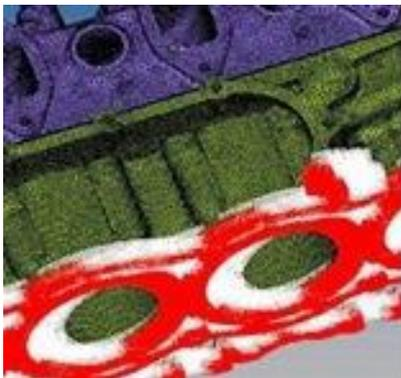
Figure 1. Boundary Conditions for Full Bank analysis
