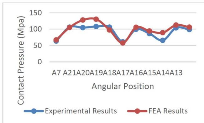
Comparison of contact pressure at cylinder 2 combustion bead
