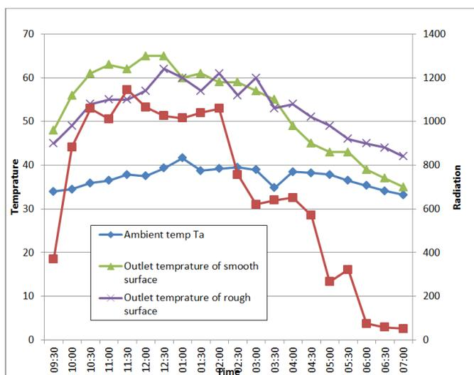
**Figure 4.** Comparison of outlet air temperature with time and radiation
