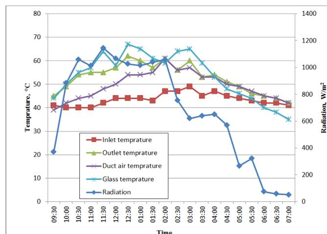
Figure 2. Variation of temperature with time at various locations in RH
