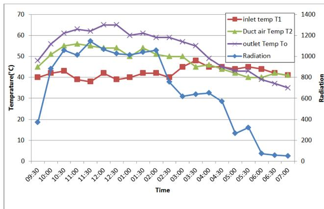
**Figure 3.** Variation of temperature with time at various locations in SH
