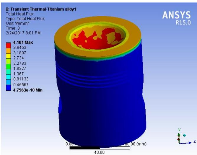
d) Titanium alloy total heat flux distribution
