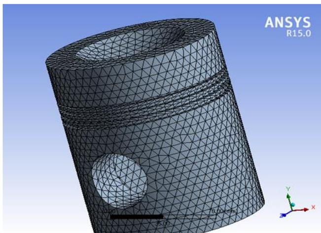
Figure 2.4 Meshing of Piston
