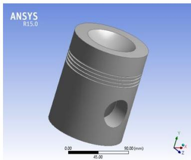
Figure 2.1 Model of the piston
