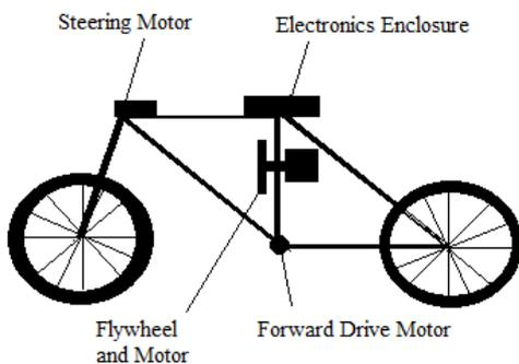
The flywheel design employs a flywheel which rotates about an axis parallel to the bicycle's frame. This design models the bicycle as a pendulum with a fixed pivot where the bicycle wheels meet the floor. As the bicycle begins to fall to one side, a motor mount to the bicycle exerts a torque on the flywheel, causing a reactionary
