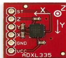
**Fig. Triple Axis Accelerometer ADXL335**
