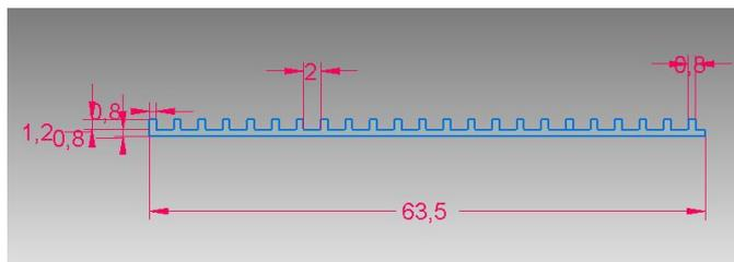
**Figure 1:** Design of a rectangular micro fin
