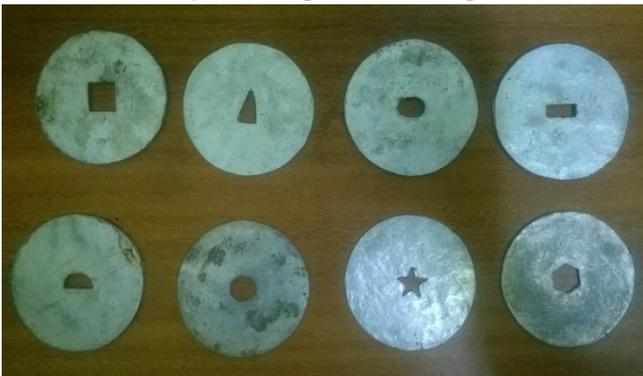
**Figure 2 :** Shapes of orifices
