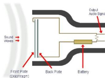
**Figure 3.** Cross Section of Microphone
