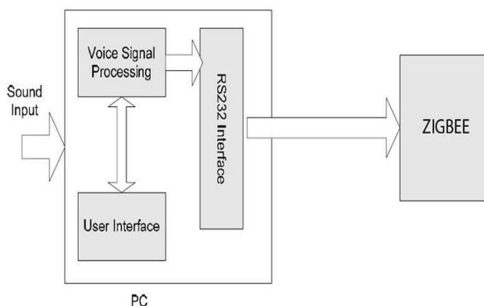
**Figure 1.** Transmitter Side
