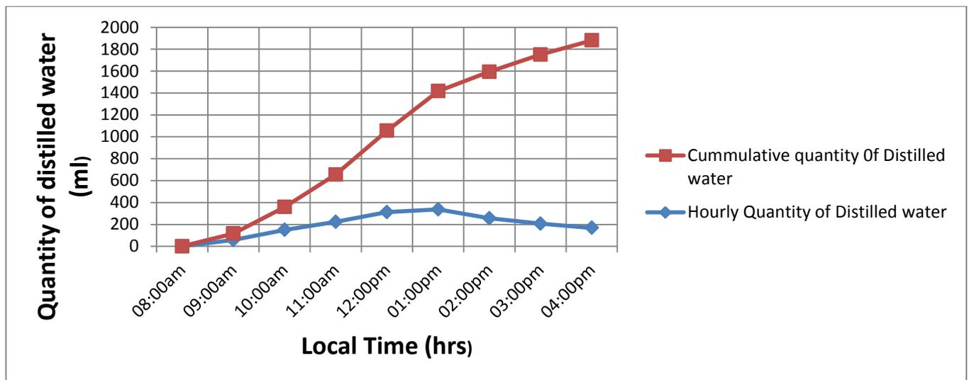
**Figure 3:** Quantity of Distilled Water Produced versus Local Time at an Average Solar Radiation of  $520.66\text{W/m}^2$  and Relative Humidity of 49.57%
