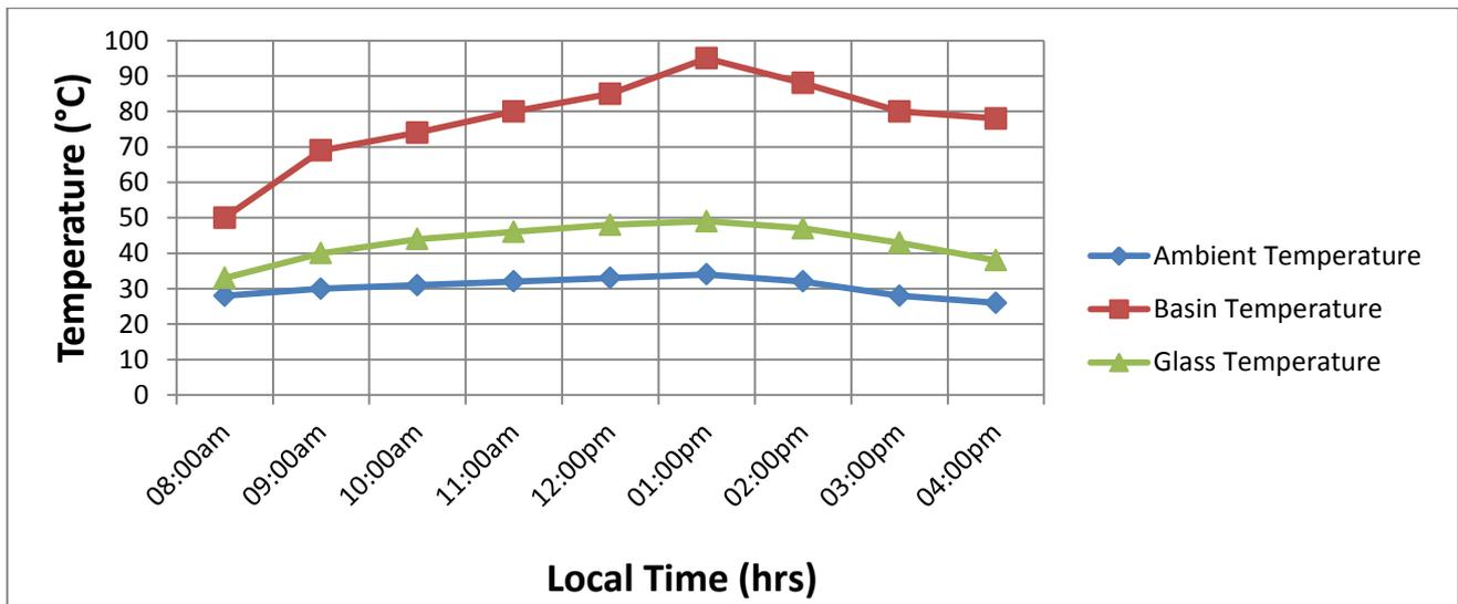
**Figure 1:** Unloaded Test Still Temperature against Local Time at an Average Solar Radiation of  $547.36\text{W/m}^2$ .
