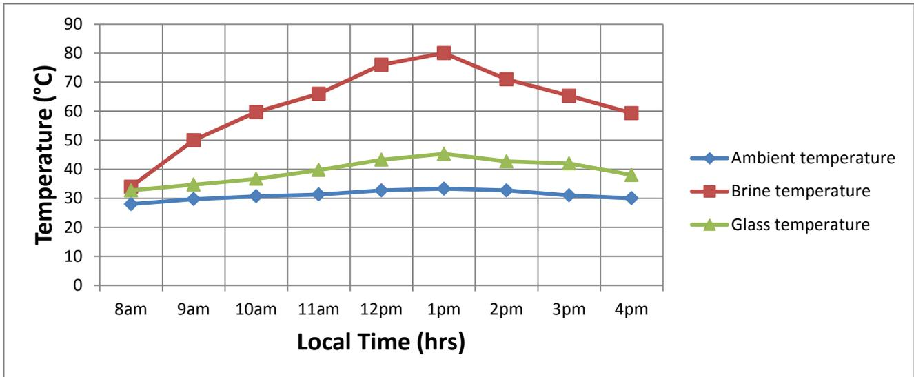
**Figure 2 :** Load Test Still Temperature against Local Time at an Average Solar Radiation of  $520.29\text{W/m}^2$  and Relative Humidity of 49.57%
