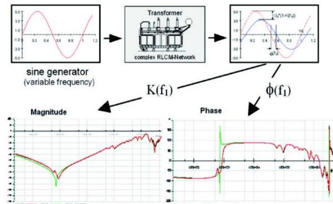
Figure 2: Basic principle of SFRA
