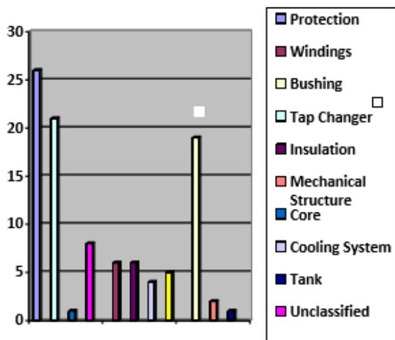
Figure 1: Failure in transformers
