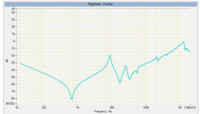
Figure 4 : HV winding between 1U and 1N at tap no:1 , with LV open
