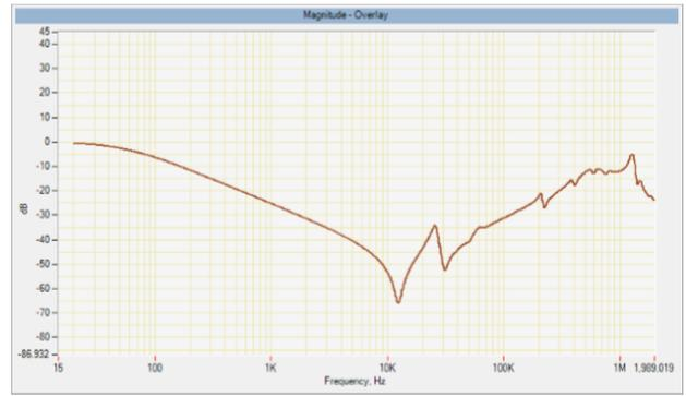
Figure 3:HV winding between 1U and 1N at tap no:1 , with LV short
