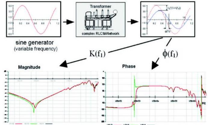
Figure 2: Basic principle of SFRA
