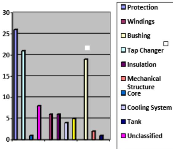
Figure 1: Failure in transformers
