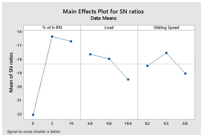
**Figure 3:** Mean of S-N ratio (wear)
