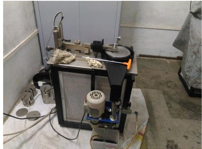
Figure 2: Pin on disc set up
