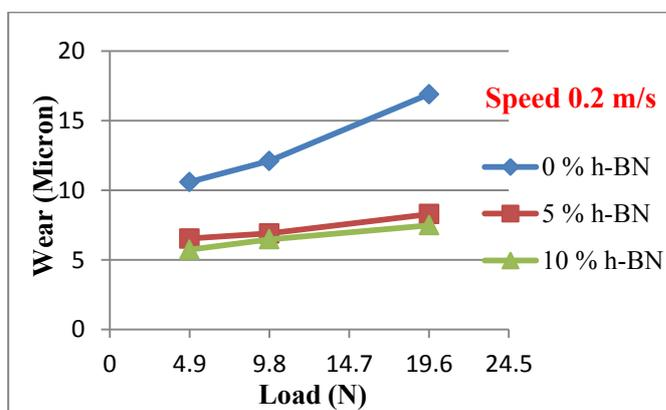
**Figure 4:** Variation of wear with load for different aluminium composite at a constant speed 0.2 m/s
