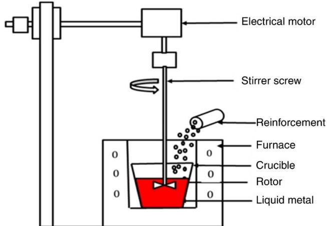
Figure 1. Stir casting set up
