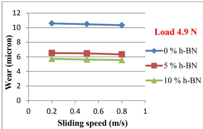
**Figure 5:** Variation of wear with sliding speed for different aluminium composite at a constant load 4.9 N
