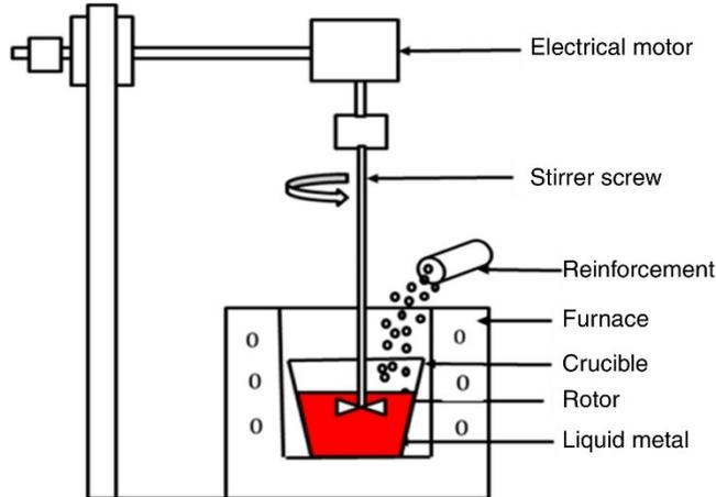
Figure 1. Stir casting set up
