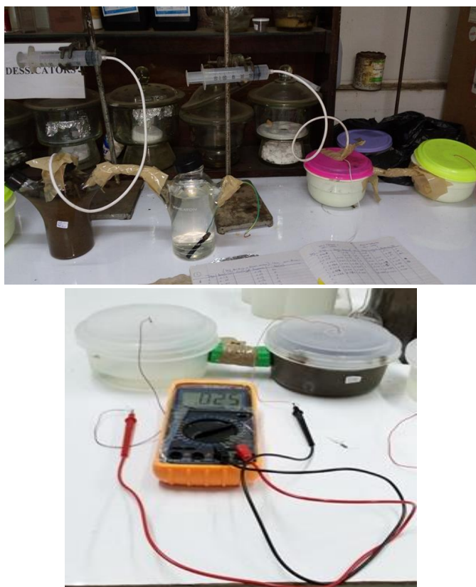
Figure 1: Set-up of H-shaped microbial fuel cells (a) open circuit with gas collection syringe (b) open circuit voltage
