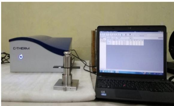
Figure 4. Thermal Conductivity Measurement
