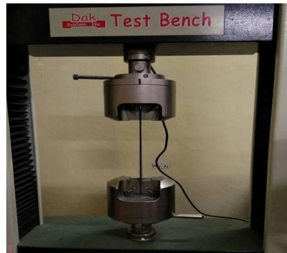
Figure 3. Tensile Strength Measurement
