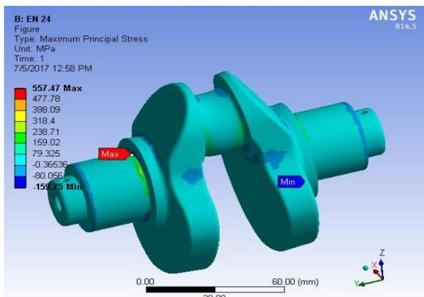
**Figure No : 13** Maximum Principal Stress (EN 24) of Crankshaft
