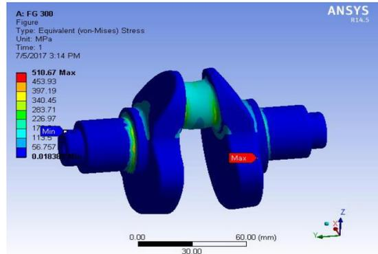
**Figure No : 5** Von Mises Stress Distribution (FG 300) of Crankshaft.
