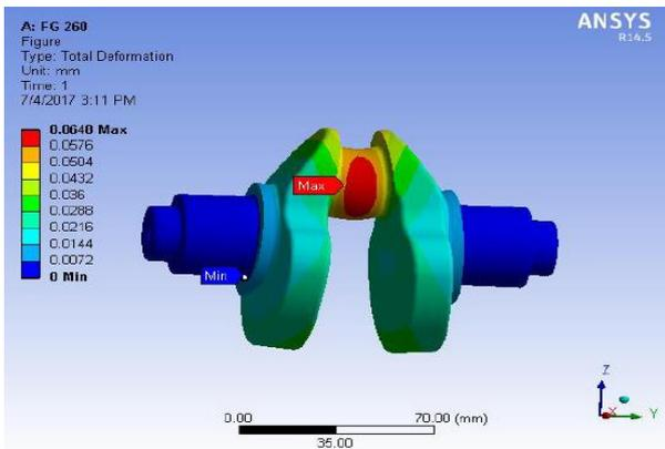
**Figure No: 3** Deformation of (FG 260 material) crankshaft
