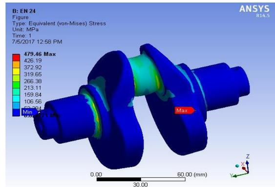
**Figure No : 11** Von Mises Stress (EN 24) of Crankshaft.
