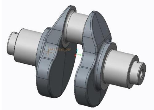
Figure No:- 1 Three Dimensional Modeling Original Crakshaft in Creo 2.0
