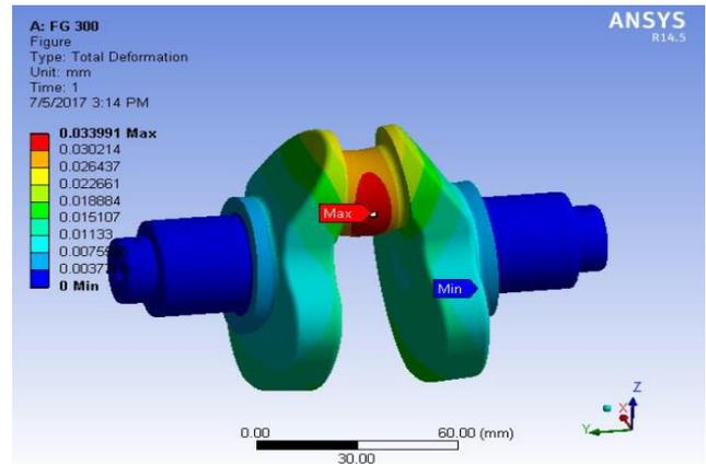
**Figure No :-6** Deformation of (FG 300) Crankshaft
