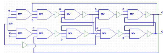
Figure 19. Proposed evaluated circuit implementation using MV gates.
