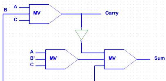
Figure.26. Proposed Full Adder Circuit Diagram with 3 MV gates
