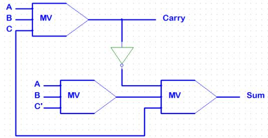
Figure.24. Full Adder Circuit Diagram with 3 MV gates[11]
