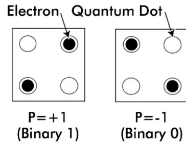
**Figure.1.** QCA cells showing how binary information is encoded in the two fully polarized diagonals of the cell[6].
