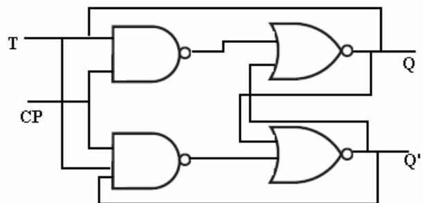
**Figure 16.** Conventional T Flip Flop
