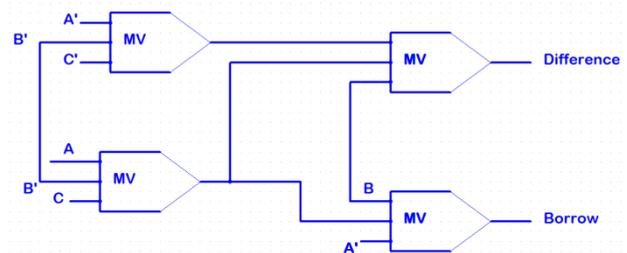
Figure.21.Full Subtractor Circuit Diagram with 4 MV gates[10]
