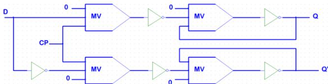
**Figure 13.** Proposed evaluated circuit implementation using MV gates.
