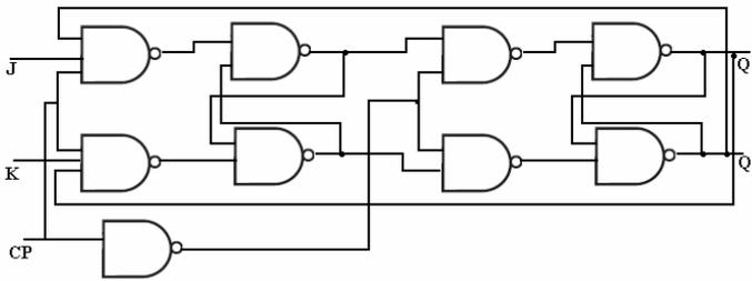
Figure 17. Conventional Master Slave JK Flip Flop
