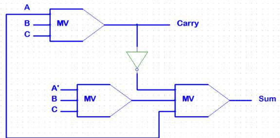
Figure.25. Proposed full Adder Circuit Diagram with 3 MV gates. Also, the circuit diagram for the corresponding circuit is shown in Fig.26.
