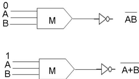
Figure.5. Structure of NAND and NOR complete gates
