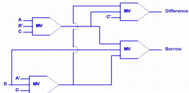
Figure.20. Full Subtractor Circuit Diagram with 4 MV gates[10]
