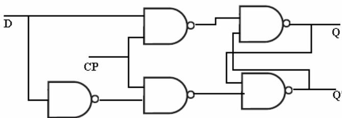
**Figure 12.** Conventional D Flip Flop
