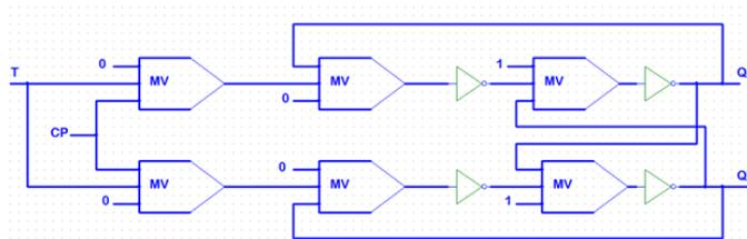
Figure 18. Proposed evaluated circuit implementation using MV gates.
