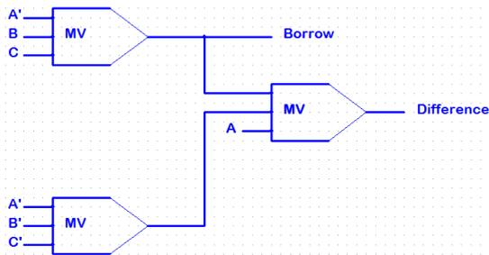
Figure.22. Full Subtractor Circuit Diagram with 3 MV gates
