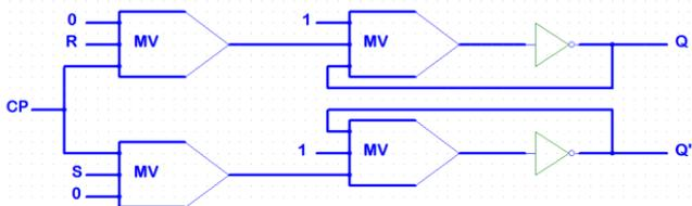
**Figure 11.** Proposed evaluated circuit implementation using MV gates.
