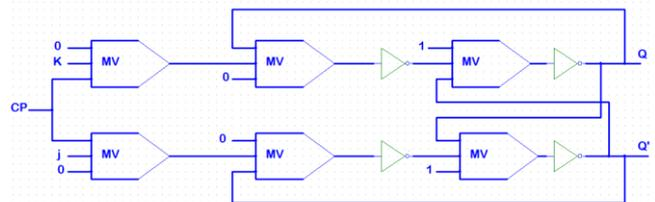
**Figure 15.** Proposed evaluated circuit implementation using MV gates.
