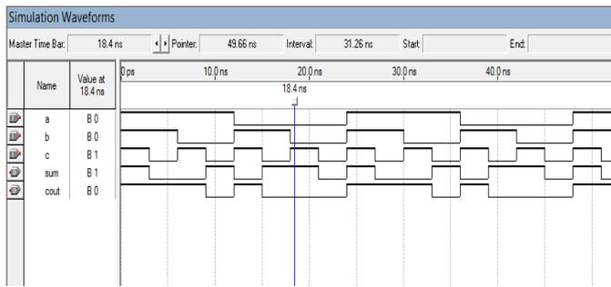
**Figure.27.** Proposed Full Adder Circuit using using Quartus II simulator.
