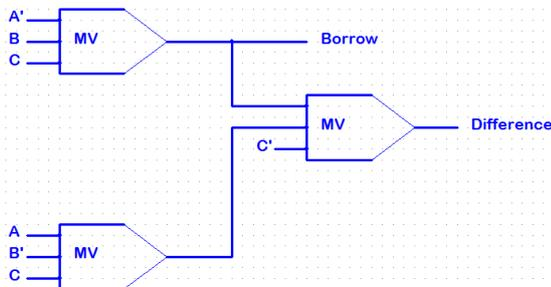
Figure.23. Full Subtractor Circuit Diagram with 3 MV gates
