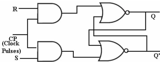
**Figure 10.** Conventional RS Flip Flop
