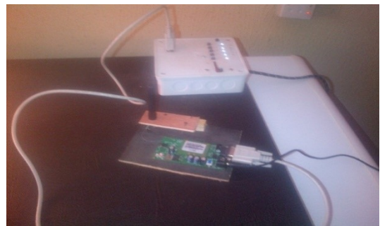
Figure 6. GSM module connected to microcontroller unit
