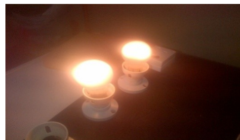
Figure 7. Lamp A and Lamp B on with _LA1LB1 command
