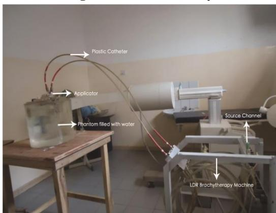
**Figure 10: Experimental Setup**
