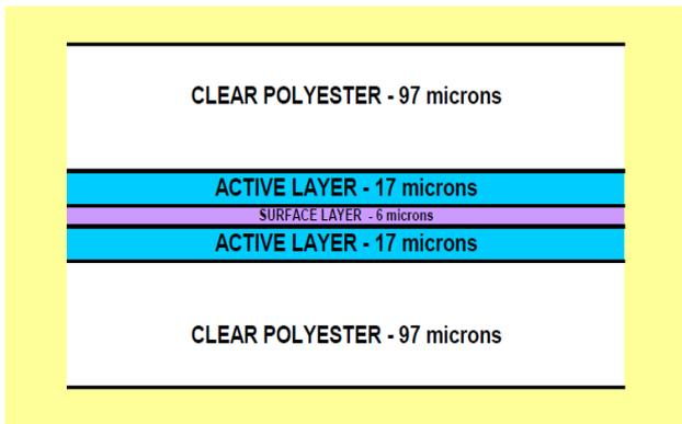
**Figure 2 :** Configuration of Gafchromic EBT Dosimetry Film
