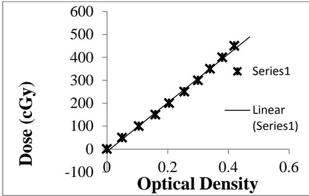
**Figure 12 :** Calibration Curve
