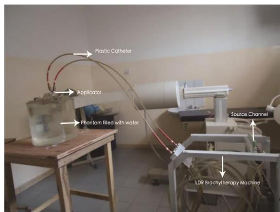
**Figure 11 :** Experimental set-up showing plastic catheters connected from the phantom to the LDR-Brachytherapy machine with Gafchromic films inserted into the rectal and bladder compartments of the phantom.
