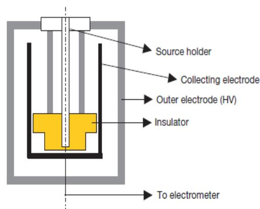
**Figure 1.** Basic design of a brachytherapy well type chamber
