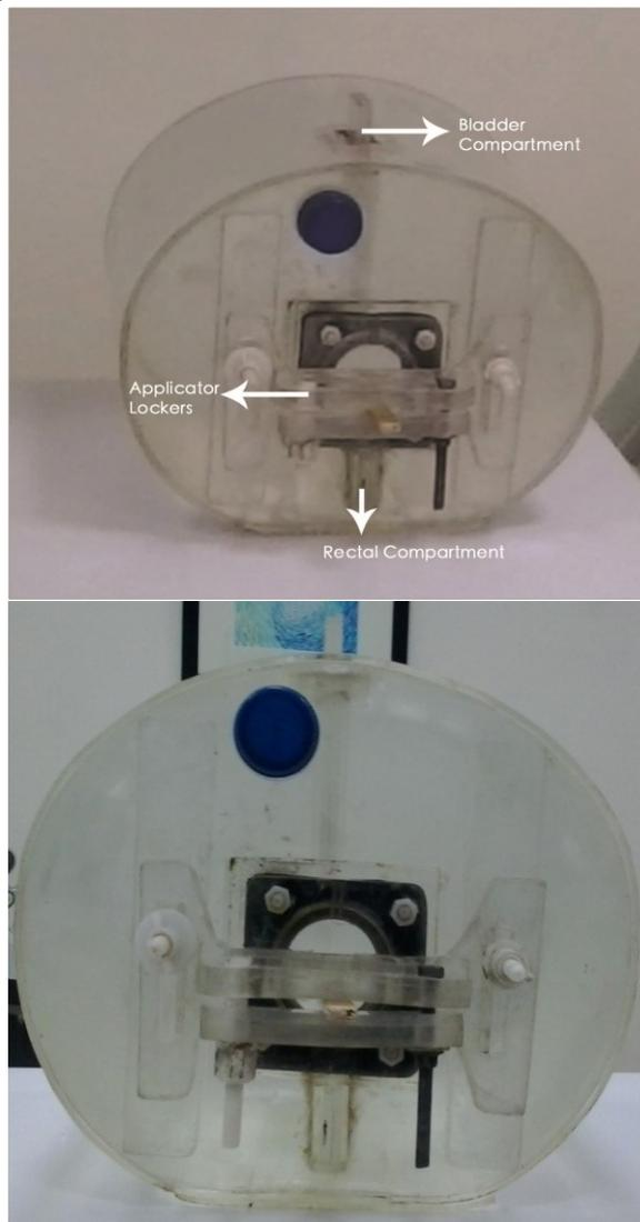
Figure 1: Built Cervix Phantom
