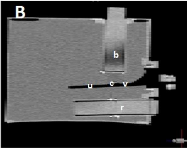
Figure 2 CT images of constructed phantom; A in transverse axial plane and B in sagittal plane.
