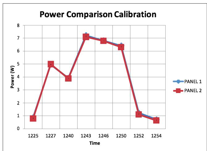
Figure 6: Power output for Panel 1 and Panel 2, both without any cooling methods applied
