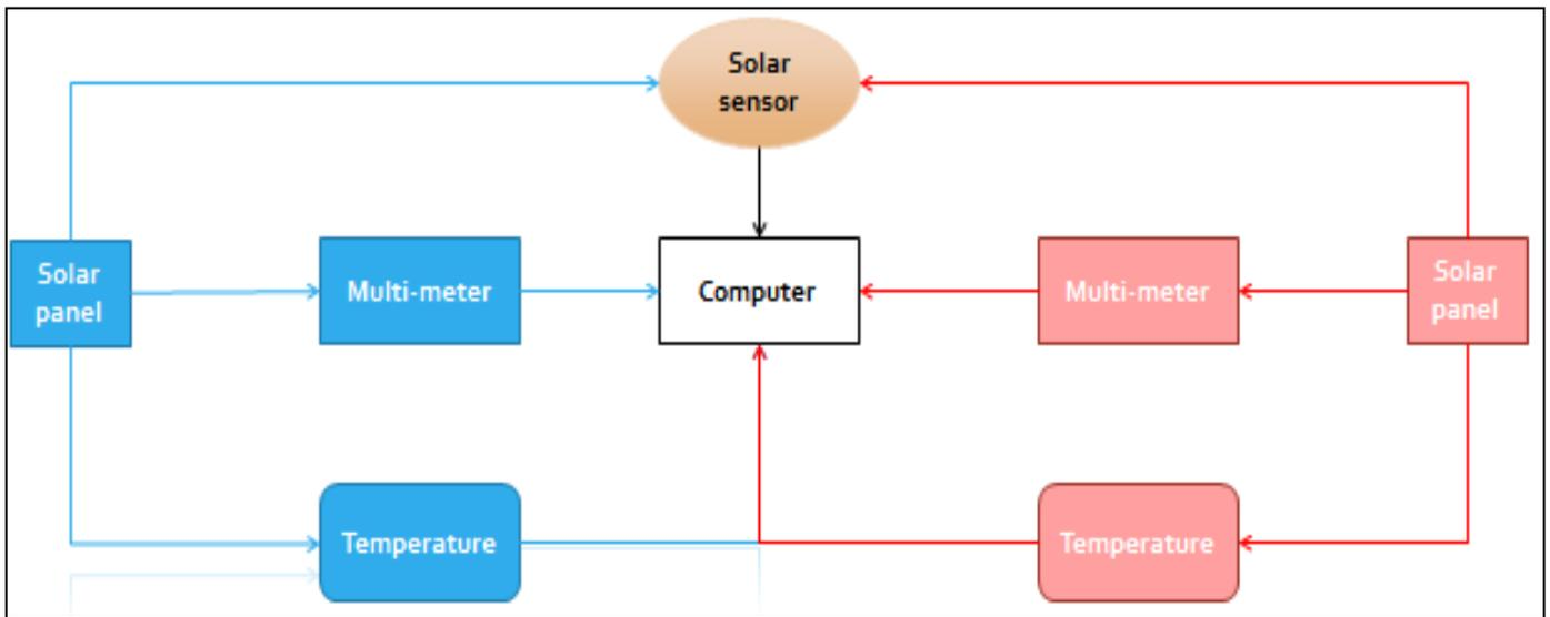
Panel 1 was labeled with blue colored tape, indicating the panel with back plate cooling method applied and
