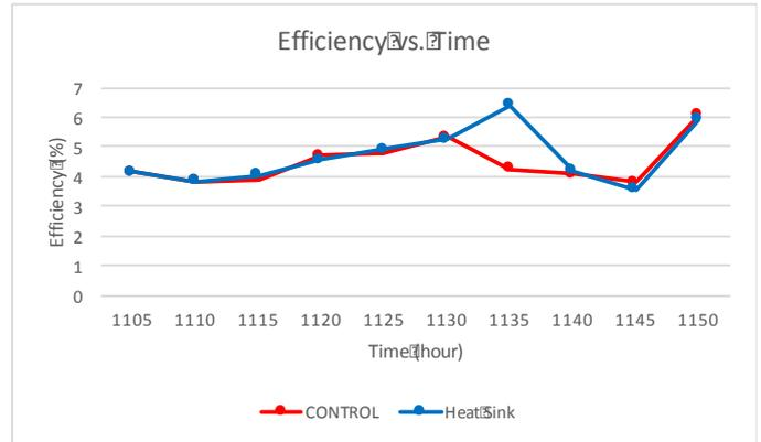
Figure 10: Panel Efficiency vs time for heat sink cooling method
