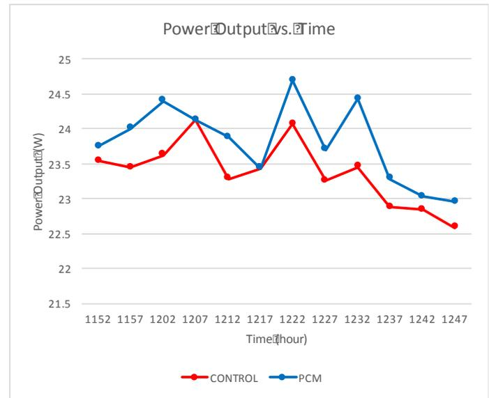
Figure 11: Power output vs. time for PCM cooling method
