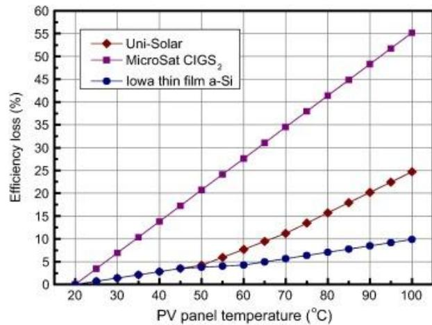
Figure 3: Efficiency loss of solar panel vs. panel temperature [8]
