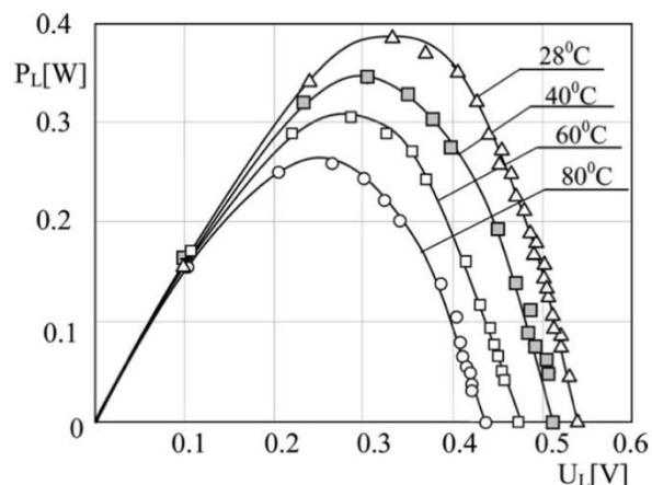
Figure 4: Power output of silicon solar cell at various temperatures [3]
