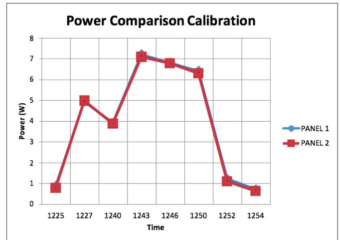
Figure 6: Power output for Panel 1 and Panel 2, both without any cooling methods applied
