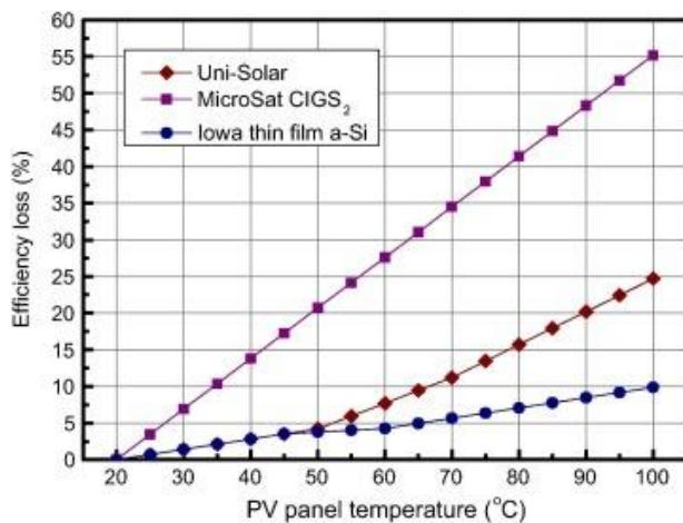
Figure 3: Efficiency loss of solar panel vs. panel temperature[8]
