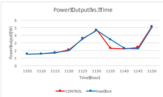
Figure 9: Power output vs. time for heat sink cooling method
