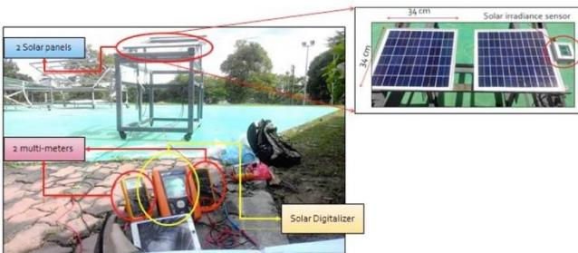
Figure 8: View of the test setup
