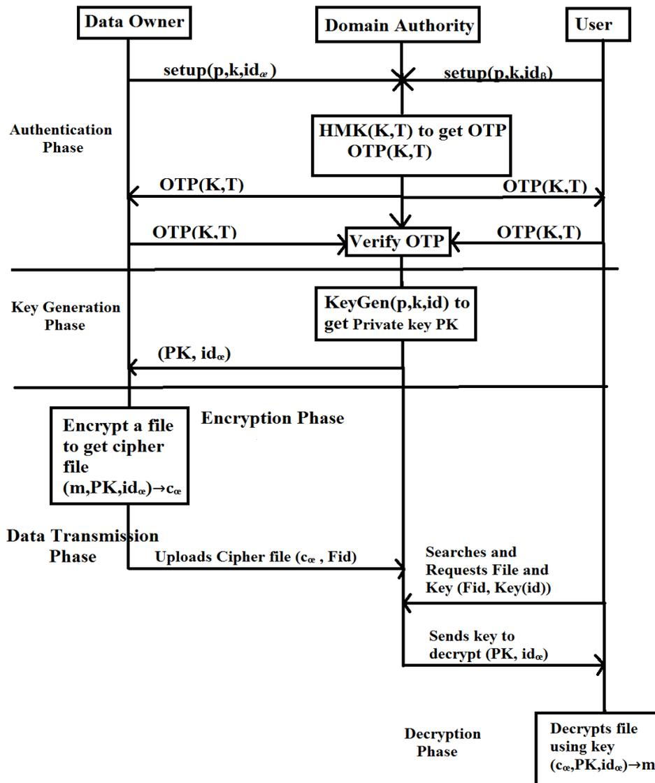
**Figure 3 : Flow of Mechanism of Proposed System**
