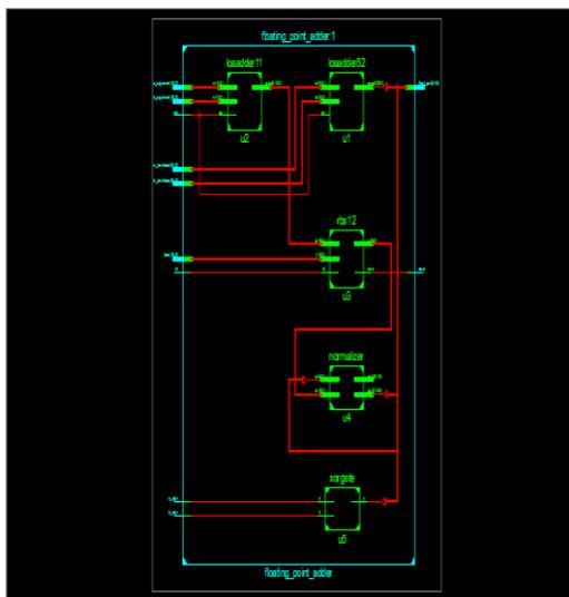
Figure 5 RTL Schematic of Inexact Double Precision Floating Point Adder
