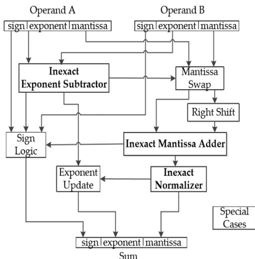
Figure 4. The Inexact FP adder architecture
