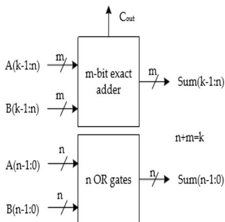
**Figure 3.** The revised LOA adder structure
