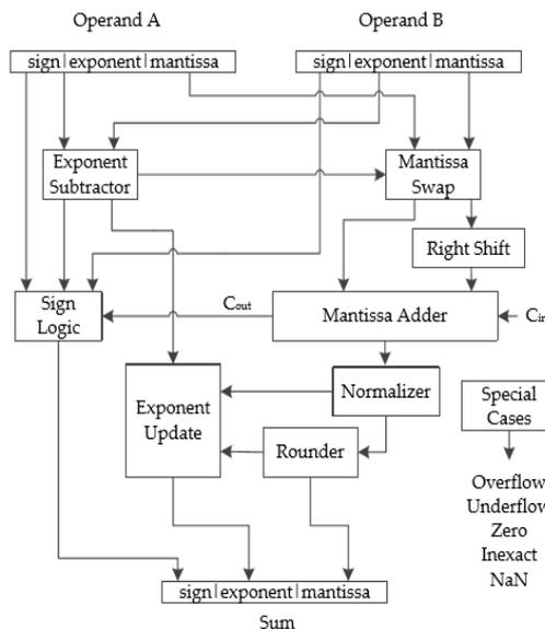
Figure 2. The accurate FP adder architecture
