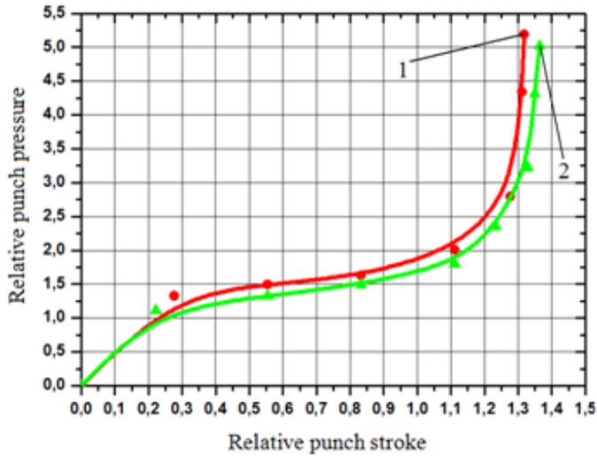
**Figure 4.** The relative punch pressure vs. the relative punch stroke in single-ended (1) and double-ended (2) radial extrusion processes with mandrel
