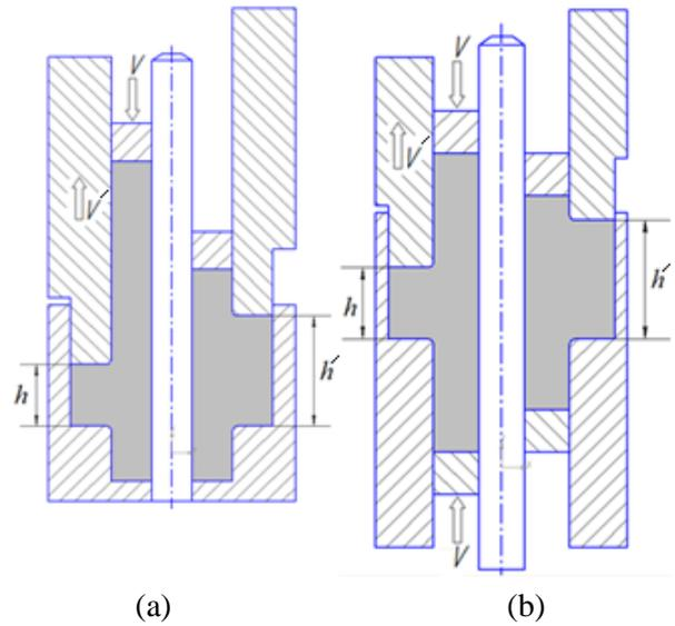
**Figure 6.** Kinematic die schemes of single-ended (a) and double-ended (b) radial extrusion processes with mandrel
