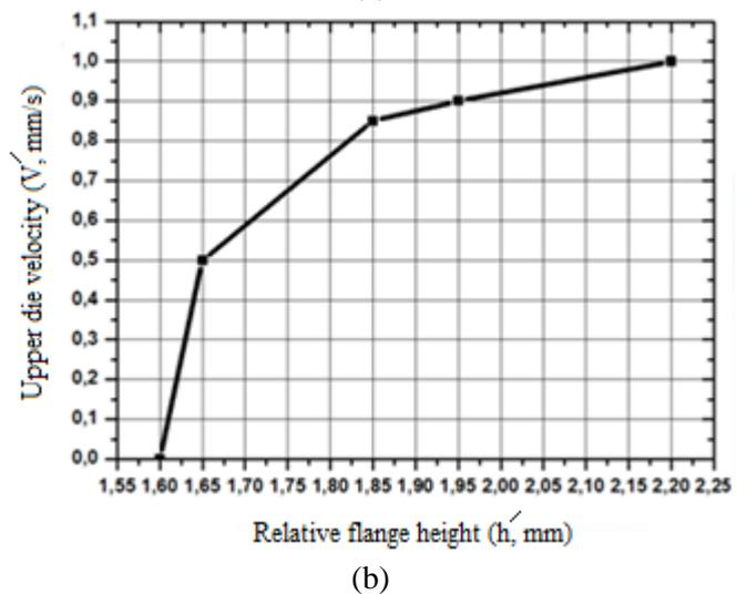
**Figure 7.** The upper die velocity vs. the relative flange height in single-ended (a) and double-ended (b) radial extrusion processes with mandrel
