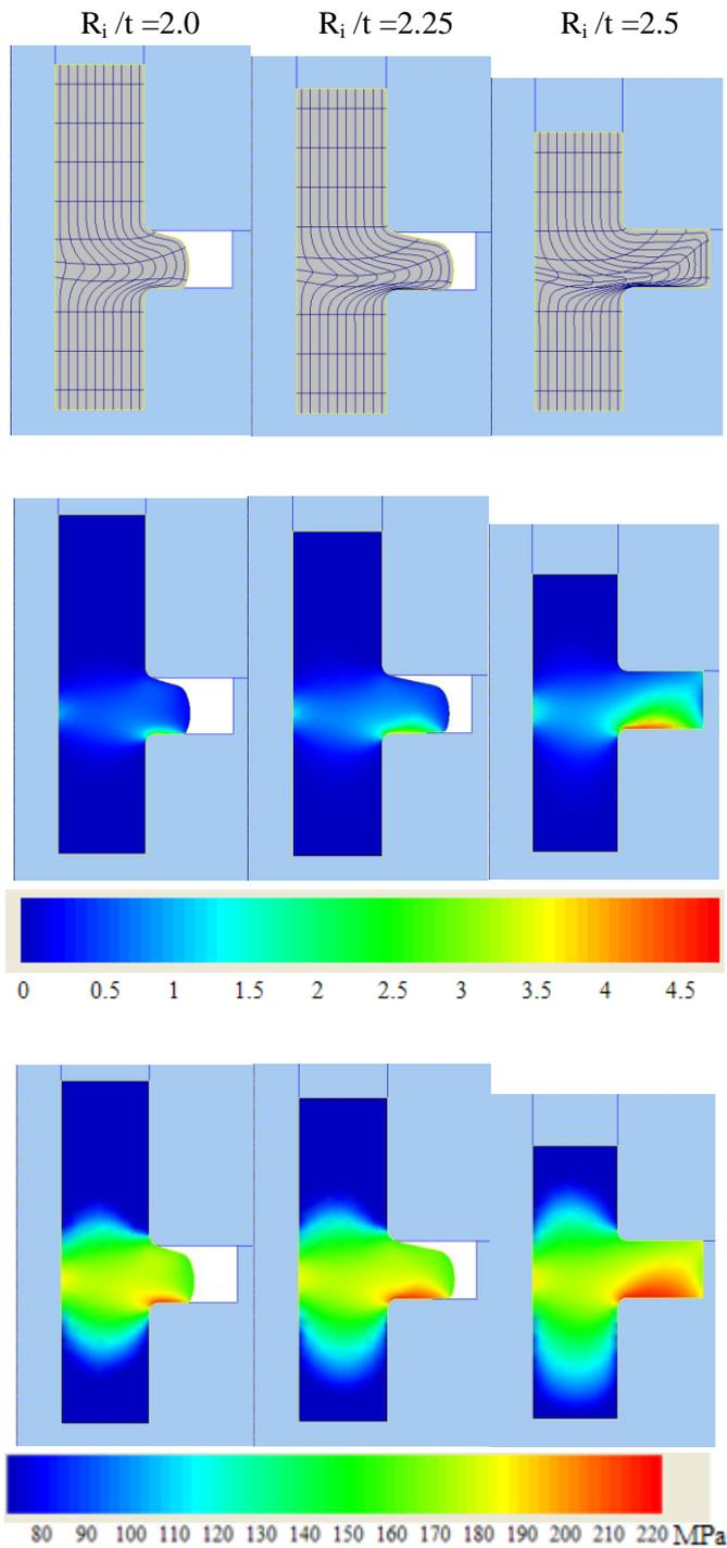
**Figure 2.** Deformation patterns or gridlines distortion (a); distributions of effective strain (b); distributions of effective stress (c) with different stages  $R_i/t$  in single-ended radial extrusion process with mandrel
