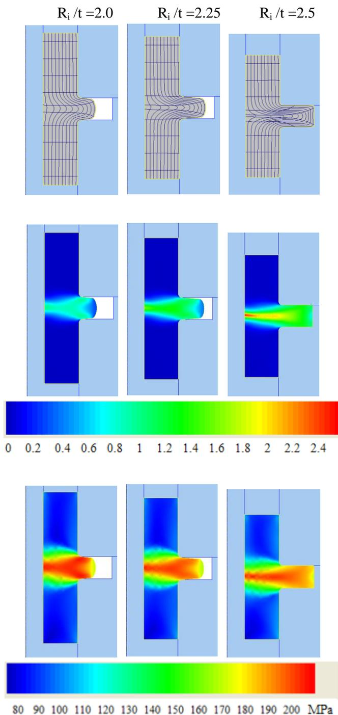
**Figure 3.** Deformation patterns or gridlines distortion (a); distributions of effective strain (b); distributions of effective stress (c) with different stages  $R_i/t$  in double-ended radial extrusion process with mandrel
