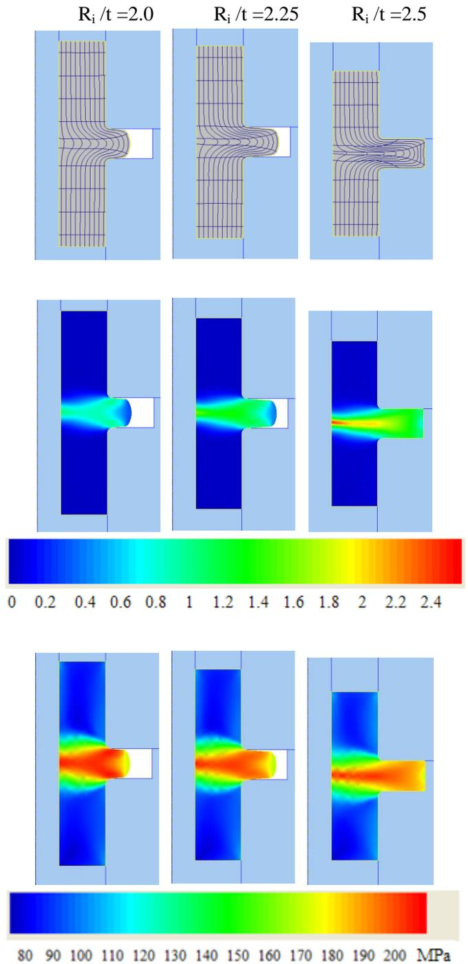
**Figure 3.** Deformation patterns or gridlines distortion (a); distributions of effective strain (b); distributions of effective stress (c) with different stages  $R_i/t$  in double-ended radial extrusion process with mandrel
