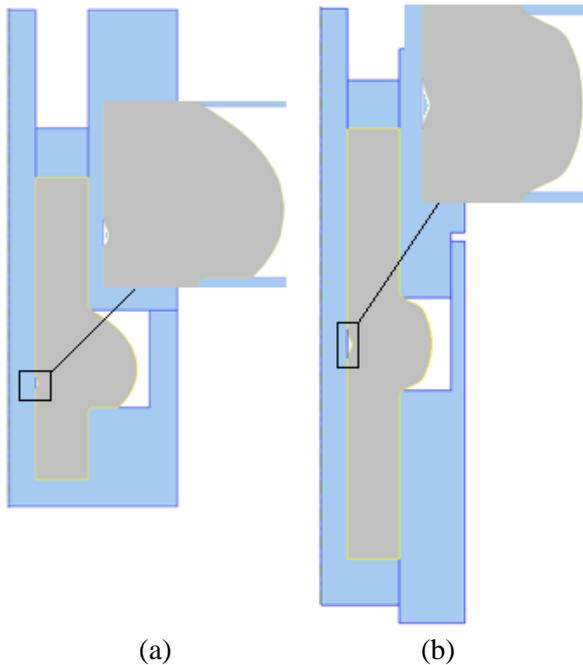
**Figure 5.** Folding defect in single-ended (a) and double-ended (b) radial extrusion processes with mandrel
