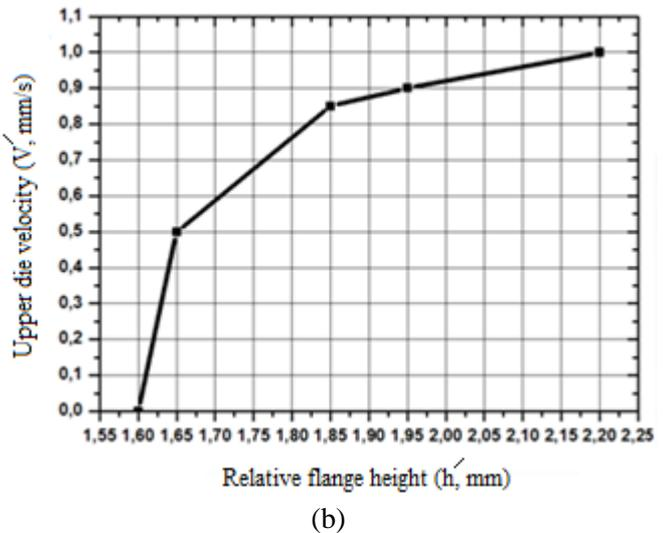
**Figure 7.** The upper die velocity vs. the relative flange height in single-ended (a) and double-ended (b) radial extrusion processes with mandrel
