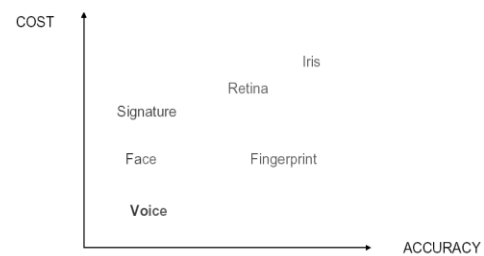
Figure 1: Comparison of different Biometric techniques
