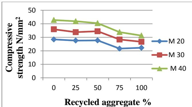
**Figure 5:** Compressive strength of concrete at 28 days
