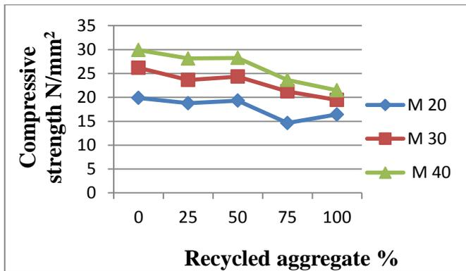
**Figure 4:** Compressive strength of concrete at 7 days
