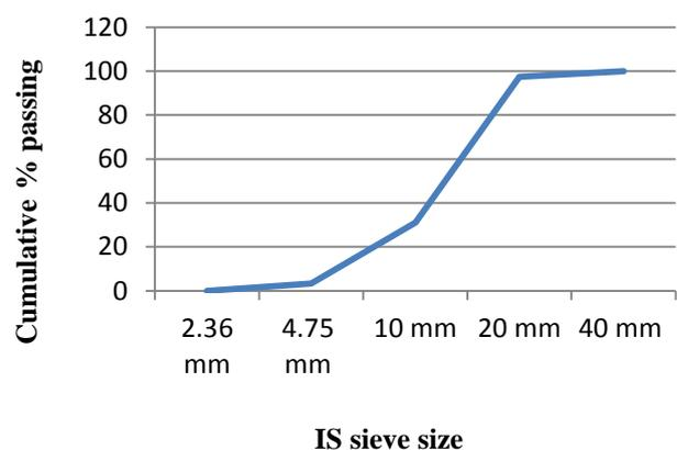
Figure 1: Gradation curve for coarse aggregates- NA
