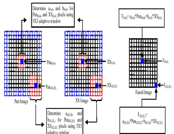
Figure 2: Construction of fused pixels using a pan and xs image
