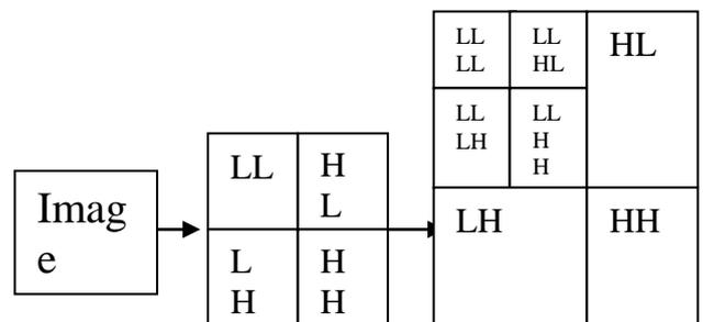
**Figure 3. Two-Level Pyramid of DWT**
