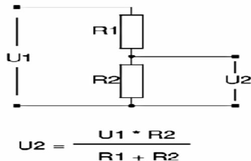
If  $R1=10K\Omega$  and  $R2= 2631.58$  ohms. Then using formula, In the figure 3, the output voltage of the voltage divider is 5v
