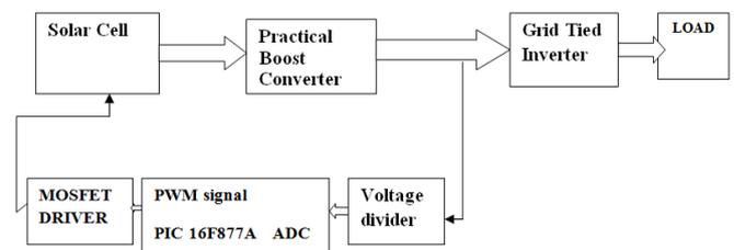
Figure 1: Block diagram of the proposed system
