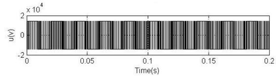
**Figure 7 :** The oscillogram of phase voltage of VSC HVDC model.
