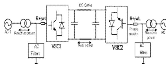
Figure 1: Block diagram of VSC HVDC model
