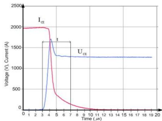
**Figure 3:** The current and voltage waveforms of real IGBT (type 5SNR).
