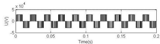
**Figure 8 :** The oscillogram of phase-to-phase voltage of VSC HVDC model.
