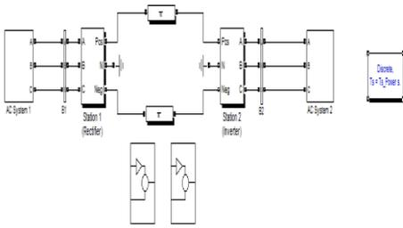
**Figure 4:** The pattern of simulation research of VSC HVDC model: Tr- transformer, F- filter, C- capacitor bank.
