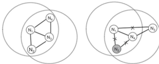
**Figure 2.** an illustration, where a failed node is shaded and a link with a cross mean that the link is down.
