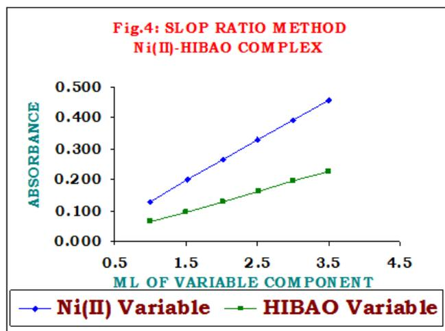
**Figure IV** : Slope ratio method.
