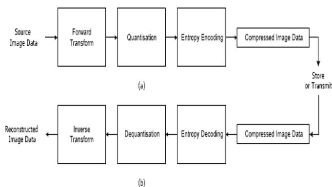
**Figure.1:** Block diagram of JPEG2000 (a) encoder (b) decoder
