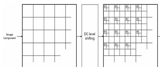
**Figure 2:** Tiling, DC level shifting and DWT of each image tile component.
