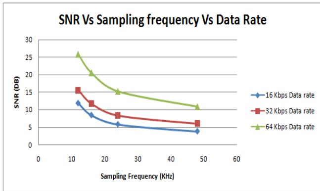
The SNR calculated at different data rates at different frequencies. Here if we increase the data rate of the CVSD system the signal to noise ratio is increases and if we increase the sampling frequency of the input signal then comparison of the comparator is decreases so signal quality at output of decoder is decreases so SNR is decreases.
