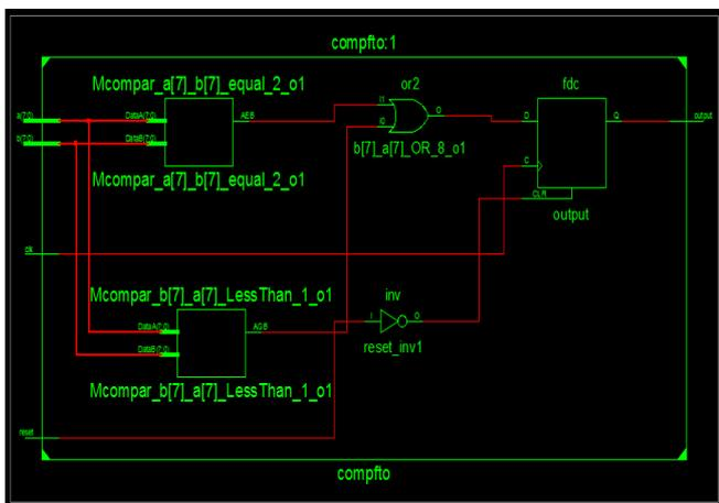
Figure 1. 8 bit Comparator RTL Schematic view in Xilinx
