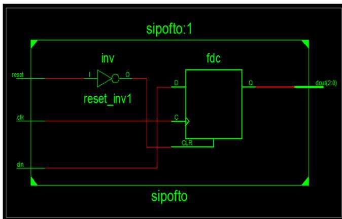
**Figure 5.** 3 bit SIPO RTL schematic view in Xilinx
