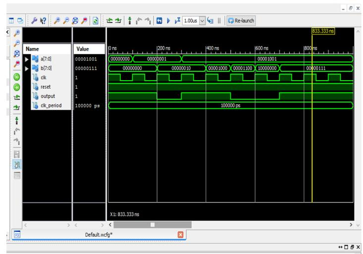
Figure 2. Test-bench simulation of 8 bit comparator created in Xilinx
