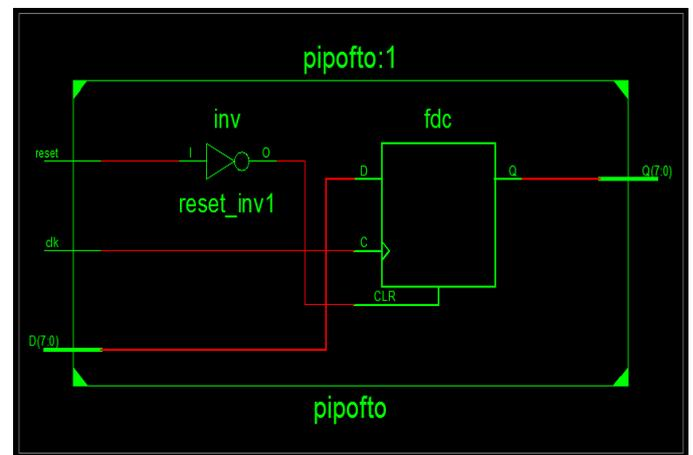
Figure 3. 8 bit PIPO RTL schematic view in Xilinx
