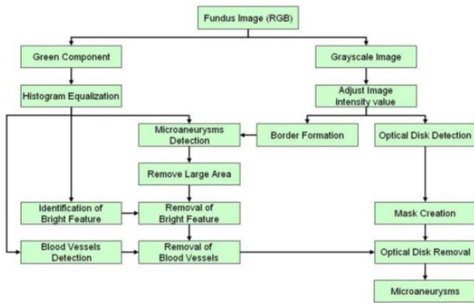
Figure 1.2 : Block Diagram for Microaneurysms Detection
