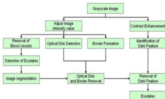
Figure 1.1. Block Diagram for Exudates Detection
