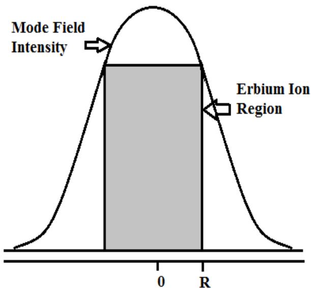
**Figure 1.** Overlap between erbium ion distribution and transverse intensity profile
