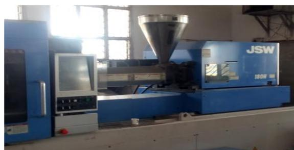
**Figure 2.** Injection Moulding Machine: JSW 180H
