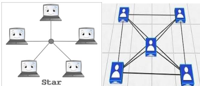
Fig. 2. Star and point to point network topology.
