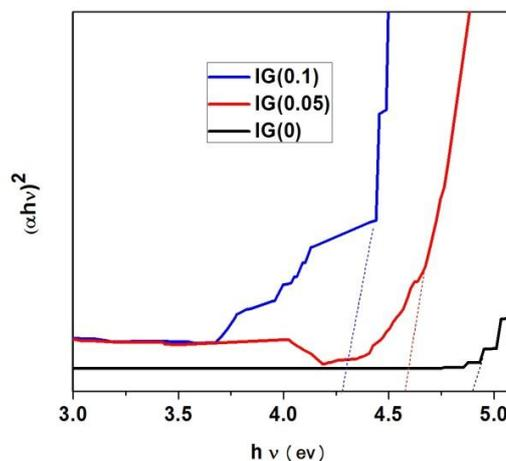
The band gap of the materials calculated using Kubelka-munk equation
