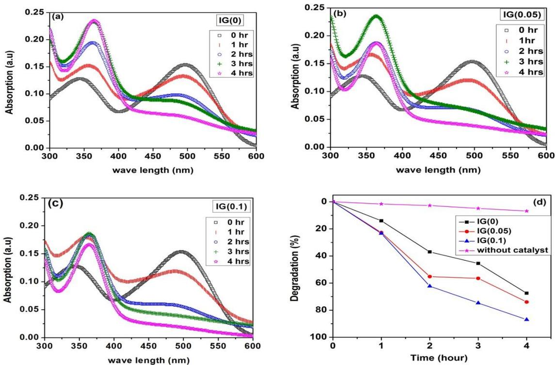
**Figure 5:** Time dependent absorption spectra of (a) IG (0) (b) IG (0.05) (c) IG(0.1), (d) Comparison of photo degradation ability of the photo catalysts
