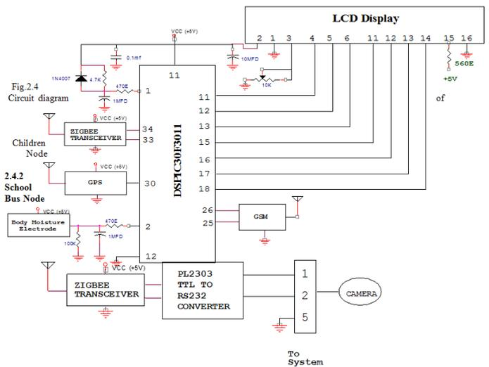
Figure 4. Block diagram of School Bus Node
