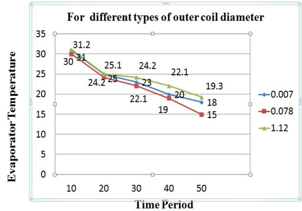
**Figure 4.** Comparison of Evaporator temp. vs Time period for different capillary tube
