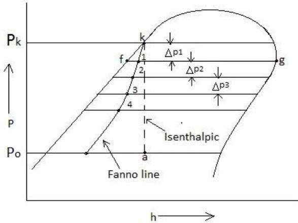
Figure 2. Incremental pressure drops in a capillary tube
