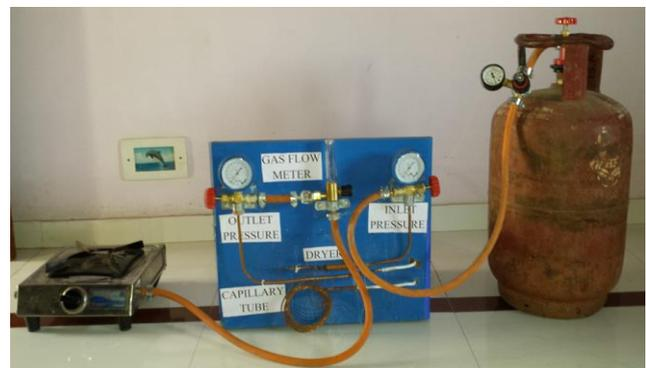
Figure1 : LPG Refrigerator Setup
