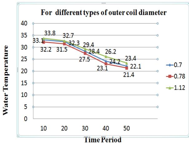
**Figure 3.** Comparison of Water temp. vs Time period for different capillary tube
