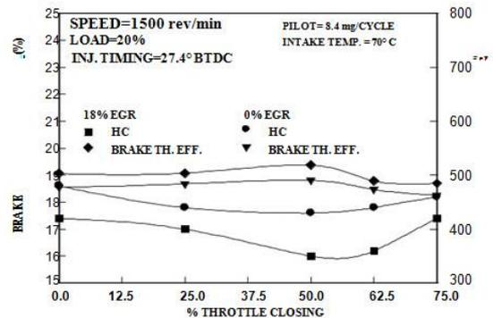
Figure 2. Effect of throttling on brake thermal efficiency and HC emissions
