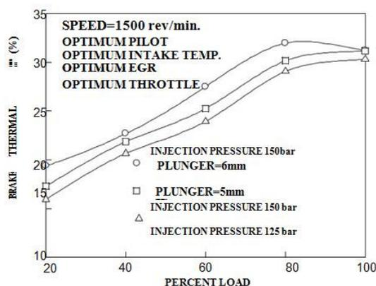
**Figure 6.** Load v/s break thermal efficiency at optimum points
