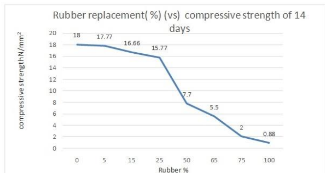
Figure 2. Rubber replacement percentage(v/s)compressive strength of 14days
