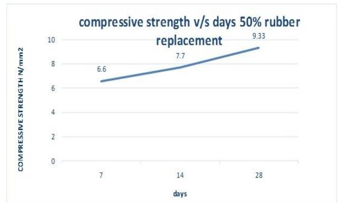
Figure 12: Compressive strength v/s days 50% rubber replacement
