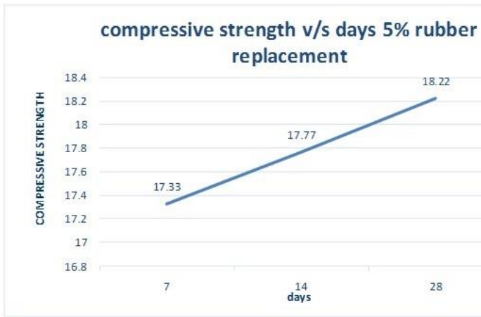
Figure 9 - Compressive strength v/s days 5% rubber replacement
