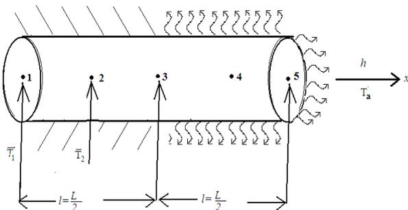
**Figure 1.** Calculation scheme for the rod at the half length of the occurring heat transfer
