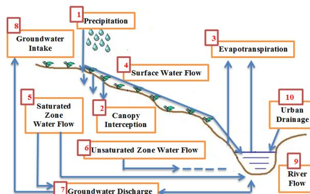
**Figure 2:** The concept of water management model in a river.
